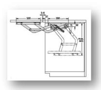
Section through the processor storage fitting
