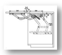
Section through the processor storage fitting
